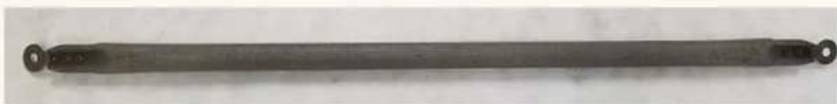
AN ORIGINAL STRUT IN STORAGE AT THE NATIONAL MUSEUM OF AMERICAN HISTORY: THE END, FLATTENED, DRILLED AND FITTED WITH ITS EYE (ABOVE), AND THE WHOLE TUBE (BELOW). ACCESSION 1983.0019; SMITHSONIAN OBJECT PHOTOGRAPHS, CC0. WEB-RESOLUTION COPIES — THE MUSEUM FILES REPLACE THEM FOR PRINT.
